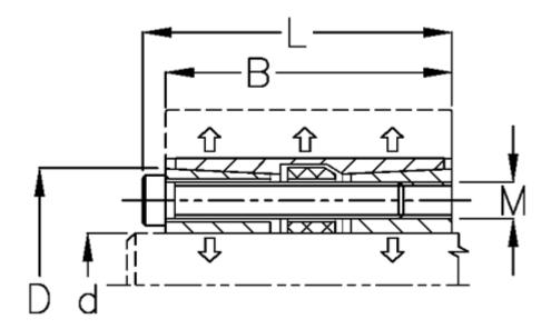
$\begin{array}{lll} \text{B mm} & = 78 \\ \text{d H8 mm} & = 60 \\ \text{D mm} & = 90 \\ \text{Fit tolerance} & = \text{Aksel h8, Nav H8} \\ \text{F kN torque} & = 220 \\ \text{L mm} & = 86 \\ \text{M mm} & = \text{M8} \\ \text{P N/mm2 surface pressure on shaft/hub} = 75 \\ \end{array}$
